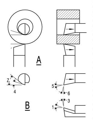
A. COMPARISON BETWEEN BORING TOOL AND CONVENTIONAL KNIFE TOOL B. TO AVOID CONFUSION FOR THOSE READERS WHO MAY ALSO READ "TOOL AND CUTTER SHARPENING" NO. 38 IN THE "WORKSHOP PRACTICE SERIES" I AM USEING THE SAME NAMES AND NUMBERS THROUGH OUT THE TEXT FOR THE VARIOUS ANGLES THAT MAKE UP THE CUTTER.
