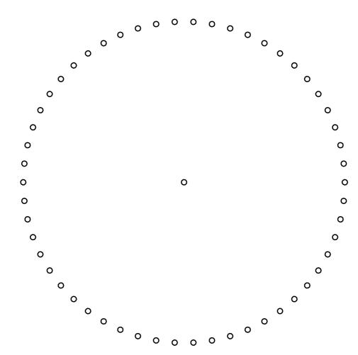
A PRINT OUT FROM A CAD PROGRAM TO ENABLE A 54 HOLE DIVISION PLATE TO BE MADE BY CENTRE PUNCHING THROUGH THE PRINT OUT ONTO THE EVENTUAL DIVISION PLATE WHICH WILL THEN BE DRILLED WITH THE REQUIRED HOLES.
